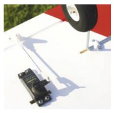
Since each aileron has its own servo, flaperon mixing is an option.
